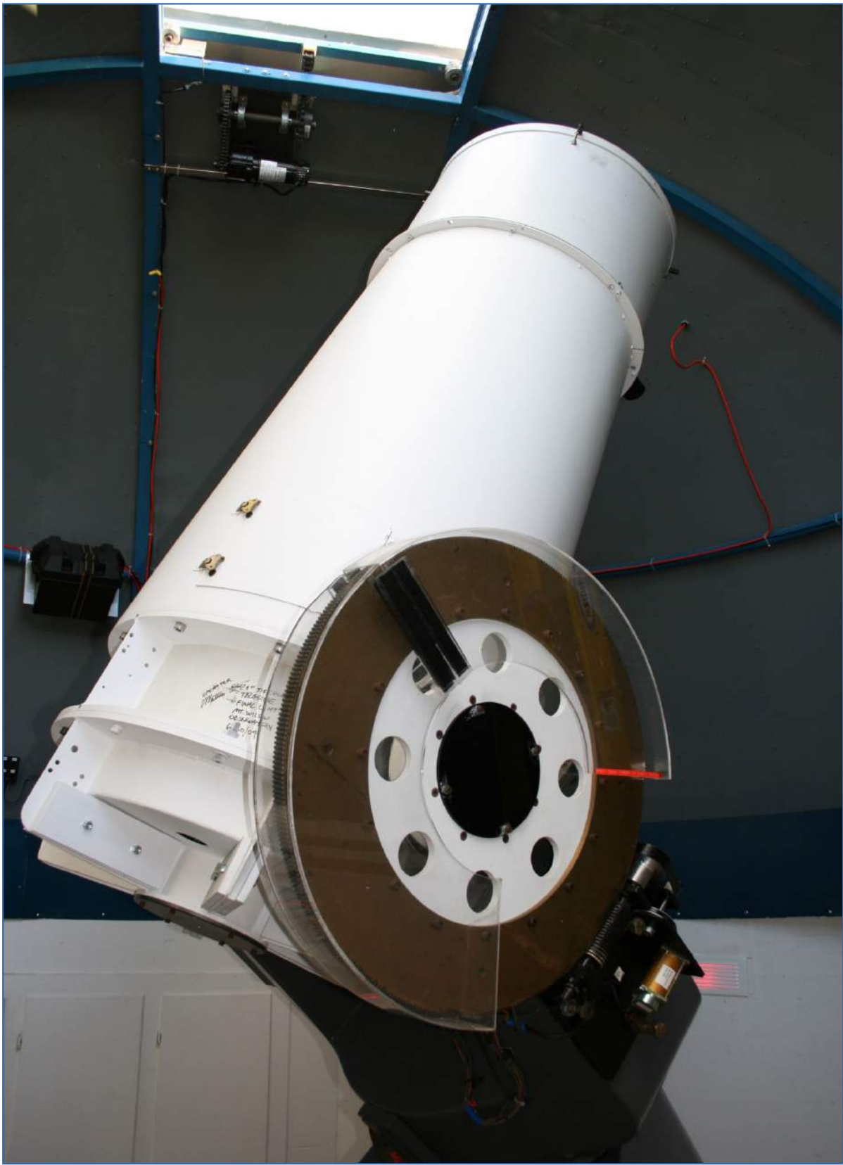
24" Telescope in F/4 Newtonian set-up
