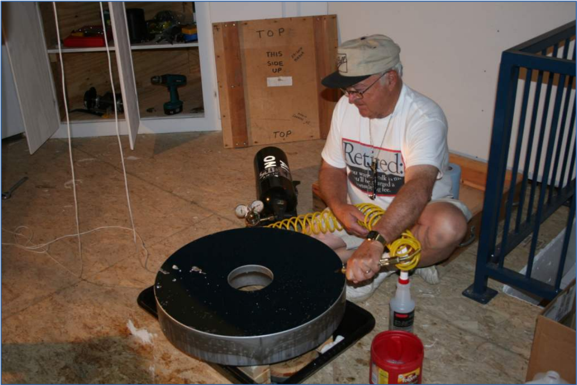
24" Primary Mirror being cleaned by Dick Gutshall
